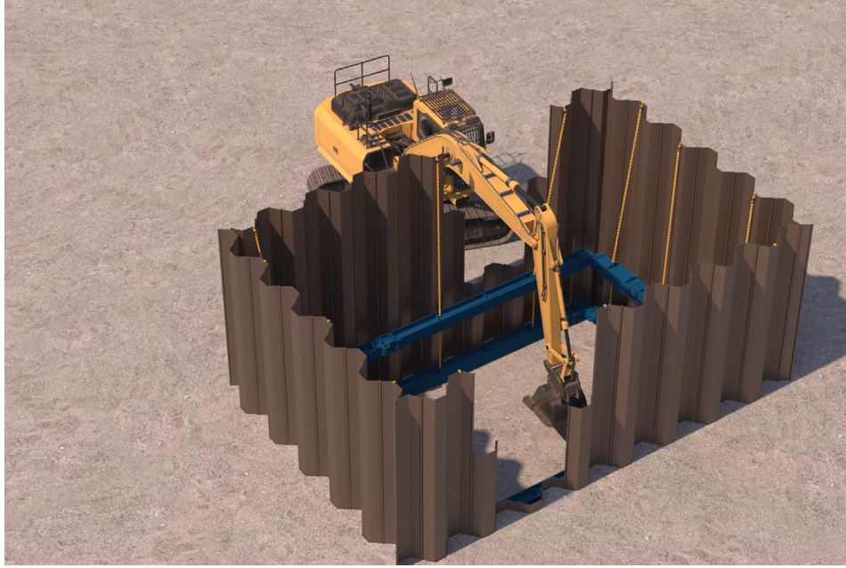
06. Install all required restraining chains before commencing excavation. Excavate beneath the lower frame to the required level of the next frame. Sheets must be driven ahead of the dig level as work proceeds (maintaining the minimum toe required by the site specific design). Alternatively the sheets may be pre-driven to their final toe-level. Ensure safe access at all times that it is required.
