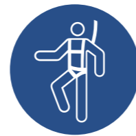
M018 Wear a safety harness
