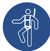
M015 Wear a safety harness
