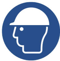
M014 Wear head protection
