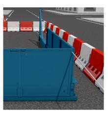
15. Prior to lifting, ensure tag lines are attached on the front and near the top of the deck on the rear, so they can be removed once installed.
