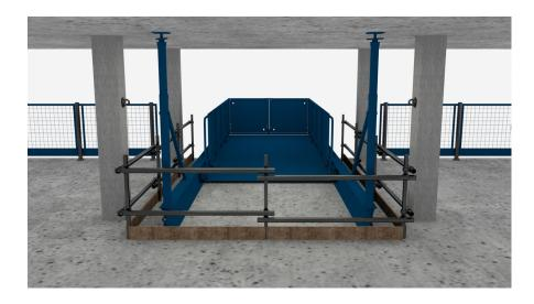
31. Check the screw jacks are tightly secured, slowly lower the crane down and disconnect the lifting chain.
