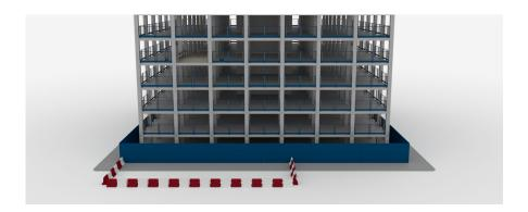
2. Create an exclusion zone at both delivery location and at the location that the platform is being installed.
