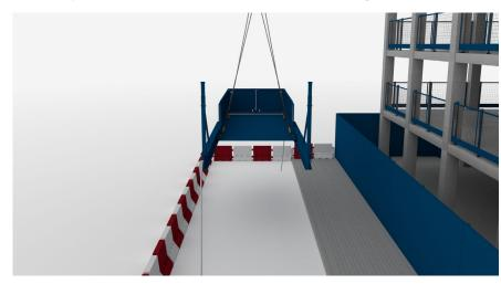
23. The deck can now be lowered to the ground to be made ready for transport or installed in a new location.
