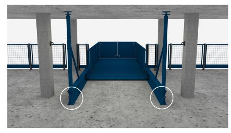
2. Once fully extended, lock into position with the shoot bolts on both sides into the outer beams.
