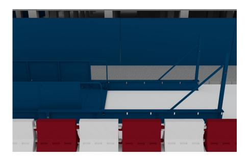
14. Prop and Brace come pre-assembled ready for installation, lift into position and secure with bolts.
