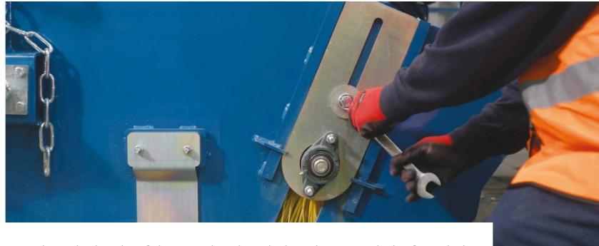
Adjust the height of the main brush with the adjustment bolt, if needed.
