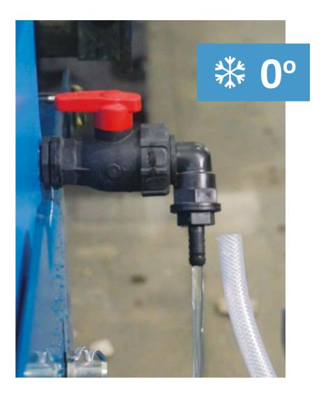
In freezing conditions, remove the hose from the water tap and drain the tank.
