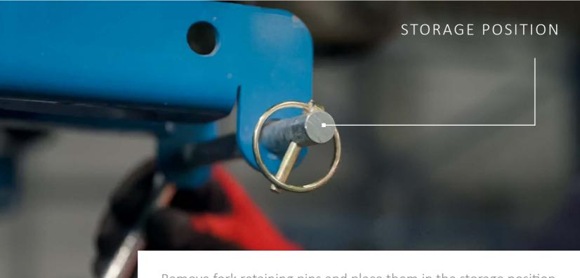
Remove fork retaining pins and place them in the storage position.
