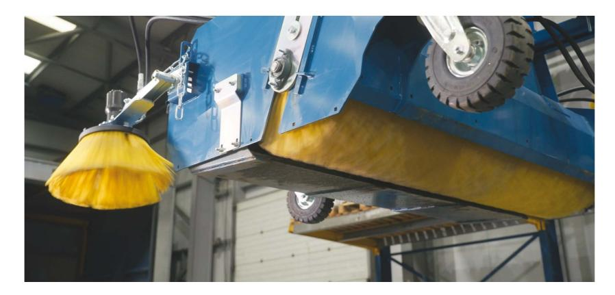
Check the brushes are visibly rotating and the hopper opens and closes fully. Never stand underneath the Powerbrush when lifted.
