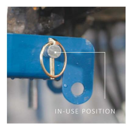
Secure the forks with retaining pins.
