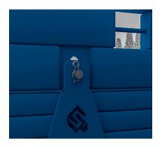
5. Attach a suitably rated 4 leg chain to the top lifting points of the extension box. Lift and carefully lower onto the base box.
