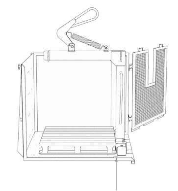
Make sure that the Crane Forks are pushed hard against the load and against the end of the fork pockets.
