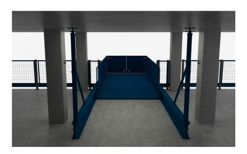
38. Remove the exclusion zone on the slab, ensuring that any gaps at the side of the deck are completed with edge protection.
