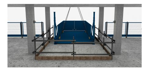
18. Manoeuvre the deck as far back into the building as possible and lower onto the slab so that both beams are flat.
