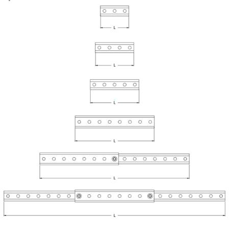
NOTE: The increments between each hole is 100mm. The resistance is 164kN.
