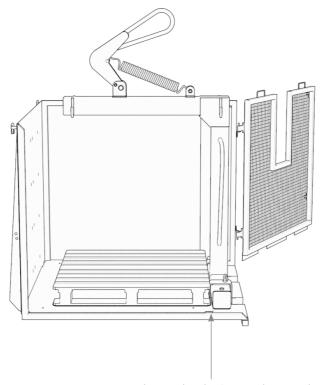
Make sure that the Crane Forks are pushed hard against the load and against the end of the fork pockets.
