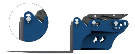
4. Measure the fork tines to ensure there is a minimum of 100mm between the base of the frame and the base of the fork tine. This applies to both fixed and floating fork variations. This 100mm allows enough space for the Autolock mechanism to lock into place as the bin is raised off the ground.
